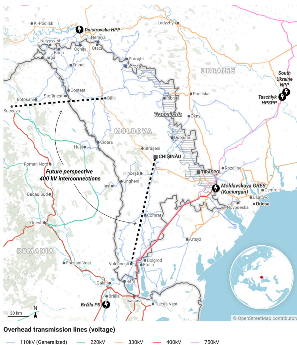
Figure 4. Map of electricity interconnections planned with Romania to bypass the Kuciurgan power plant (Moldavskaya GRES).
